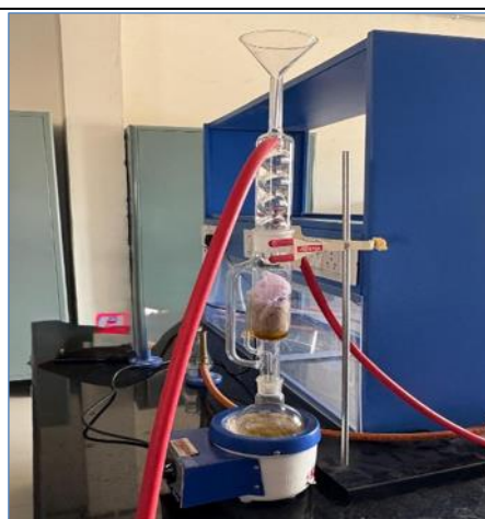
Figure 7: Soxhlet extraction using ethanol
